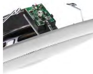
LC1-PIB fitted on the loudspeaker and showing the light conductor
